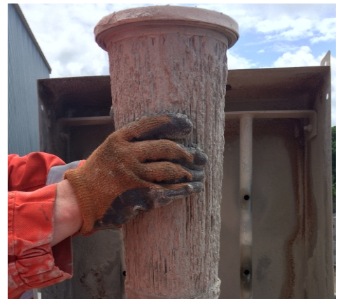
The trapped pressure from the blockage was causing the SPS pressure alarm to trigger and the PRV to lift, in order to protect the silo from damage.
