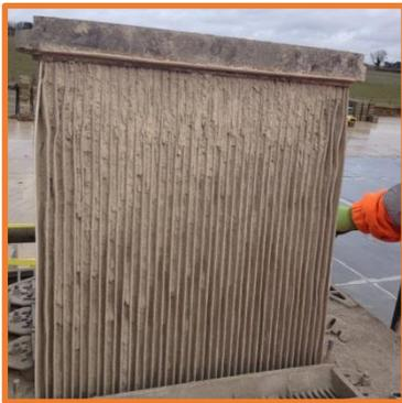
Filter cartridges in a damaged and neglected state, often completely blinded by powdered product. These pose the risk of emission issues if they burst, or if they are completely blocked they have the potential to cause serious damage to the silo. There have been several recorded incidents of blocked filter housings being blown clean off silo roofs by pressure build-up – and the dangers of heavy metal objects being thrown from height into busy work-yards or quarries do not need explaining.
